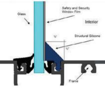
Internal testing indicates that a window with safety and security film with an attachment system provides improved protection against a would-be intruder compared to a window that has film applied without an attachment system.
